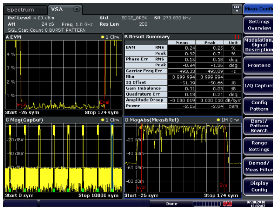
Fig. 5-5: R&S FSV-K70: Result range that exceeds the burst length
